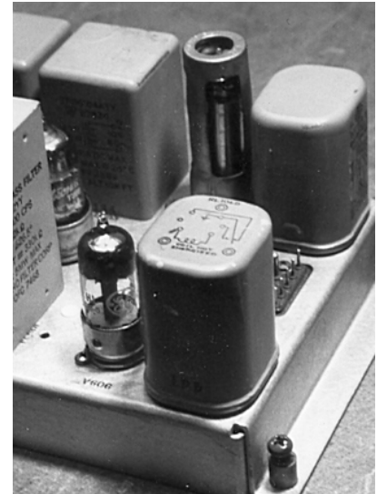
Figure 2. R-390A. Af sub-chassis, top view, front section. Squelch tube V606 (6C4) and squelch relay K602 installed.
