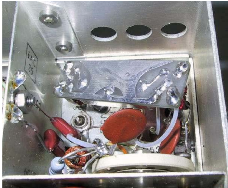
Completed Roofing Filter Mod
