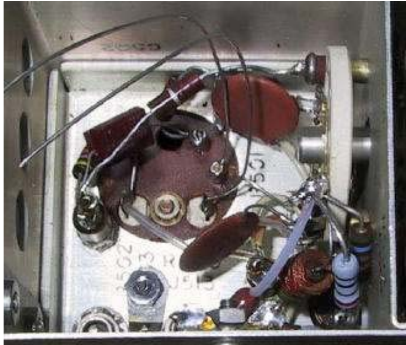
IF Deck Rear Compartment Prepared For Filter Board
