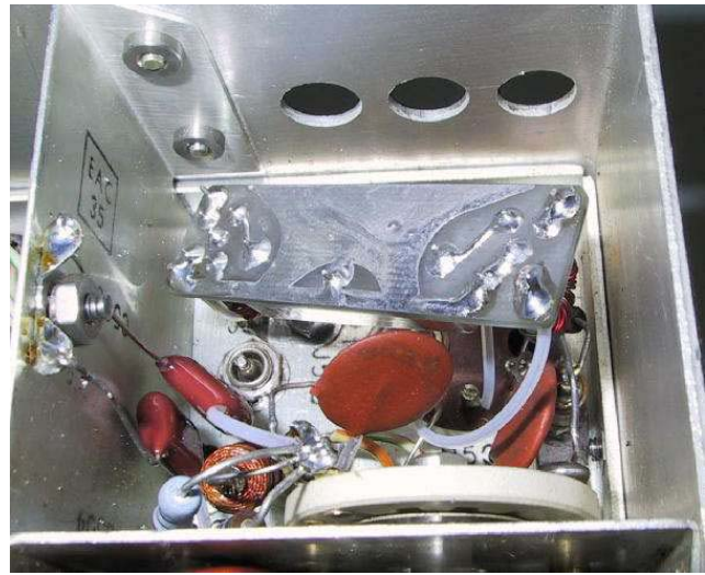
Completed Roofing Filter Mod
