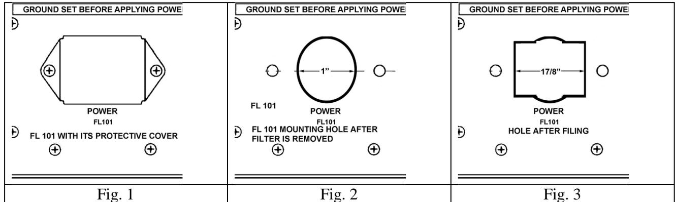
Fig. 1 shows the typical back of the receiver with the cover over FL 101. Fig 2 the hole with the filter removed and Fig. 3 the modified hole
