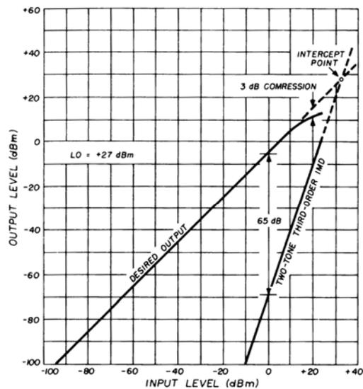
**fig 8 Third-order intercept point of high level double balanced mixer (SRA 1H) at 50 MHz is +32.5 dBm relative to the input, 3 dB compression occurs at +20 dBm and third-order IMD is suppressed 65 dB when both input signals are 0 dBm (224 mV across 50 ohms).**
