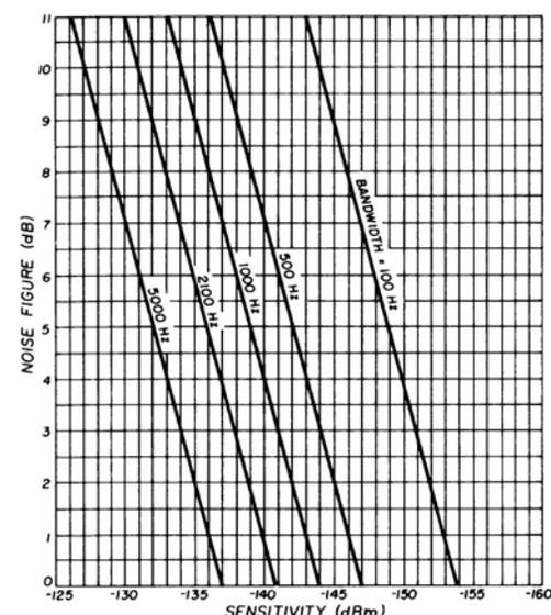
**Fig. 3. Receiver sensitivity (-dBm) vs receiver noise figure and bandwidth for unity signal to-noise ratio (signal equals noise). Add 10 dBm for a SIN ratio of 10 dB. Table 1 lists microvolt sensitivity for 50- and 75-ohm systems in terms of dBm sensitivity.**
