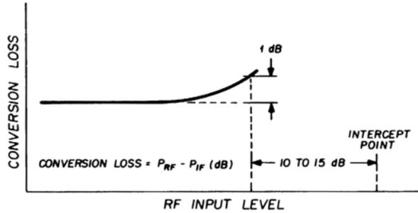
**fig. 10.** When working with double-balanced mixers, the third-order intercept point may be estimated by using the rule of thumb that the intercept point is 10 to 15 dB above the 1-dB compression point (see text).
