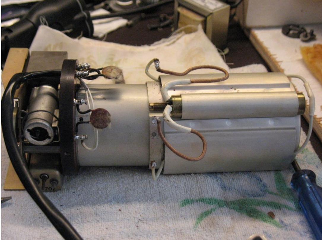
Once the heater unit is removed, you have access to the inner cover. Removing it for the first time after sitting for a long time can be quite difficult, even if the rubber seal is in good condition. As can be seen in the next photo, the seal is about a 1/4" from the base. You might try putting some silicone oil on the joint all around it and let it soak in. Sit it on the end with the electronics end up.
