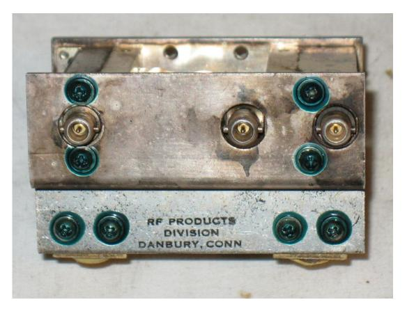
The next step is to remove the four phillips screws holding it onto the rear frame. They are pointed to in the picture below. When the last screw is being removed, the relay should be held up by one hand. The wires are still connected to it that operate the electromagnets, so be careful not to damage them. They are long enough that some repair can be done on the relay without disconnecting them.
