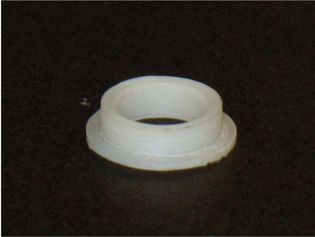
Although the spacing collar in the center on this one sticks up higher, this could still be used as it would space both the capacitor cover and the mounting bracket, and then just a flat insulating washer could be used on the top.
