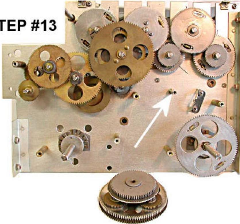
SLIDE GEAR ASSEMBLY ONTO SHAFT SMALL GEAR FACING INWARD.
