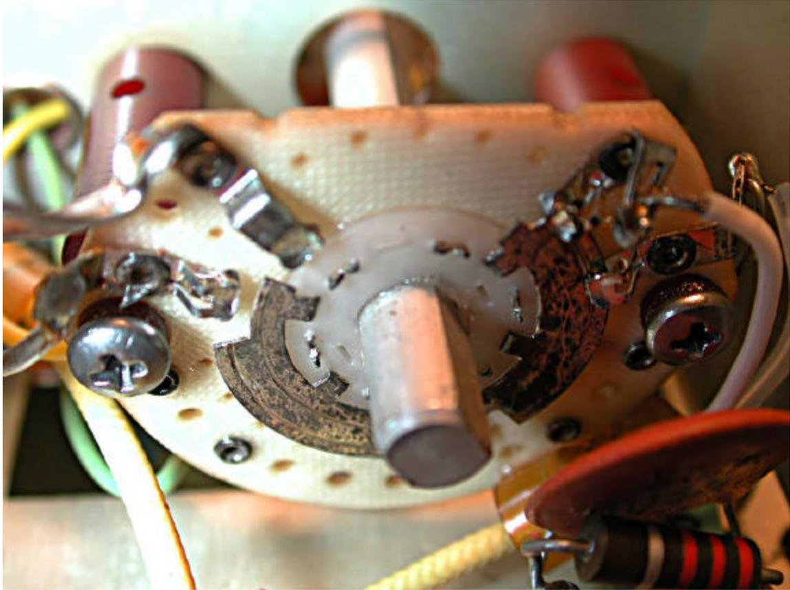
**THIS IS THE POSITION OF THE RF BANDSWITCH REARMOST CONTACTS WHEN THE DIAL IS SET IN THE 08 MHZ POSTION. THE UPPER LEFT CONTACTS SHOULD OPEN UP AS THE SWITCH IS TURNED FROM 7 MHZ TO 8 MHZ. THERE IS ONLY ONE POSITION OF THE GENEVA DRIVE THAT WILL PRODUCE THIS RESULT.**
