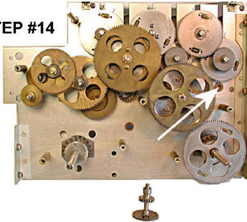
**LUBRICATE END OF SHAFT AND SLIDE INTO BRONZE BUSHING.**
