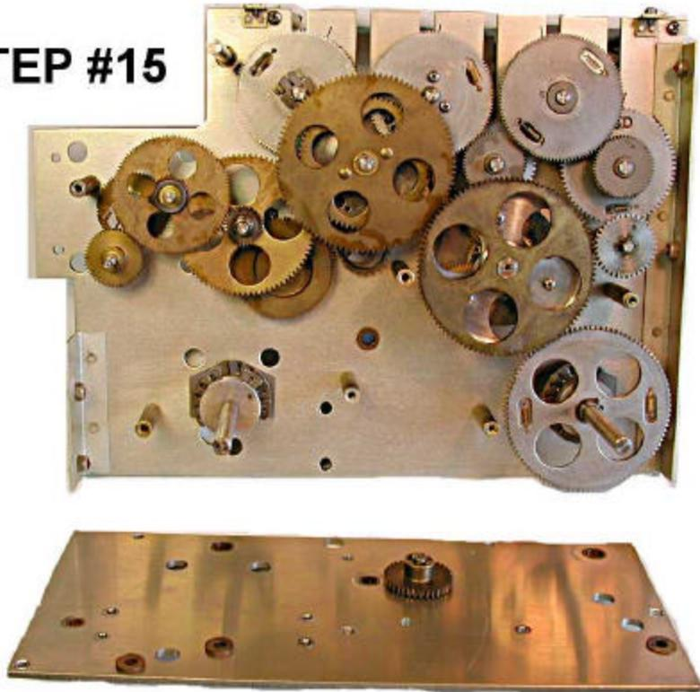
PANEL GOES ON NEXT. CAREFULLY ALIGN SHAFTS INTO BRONZE BUSHINGS ON PANEL. TIGHTEN ALL SCREWS GRADUALLY AND EVENLY.
