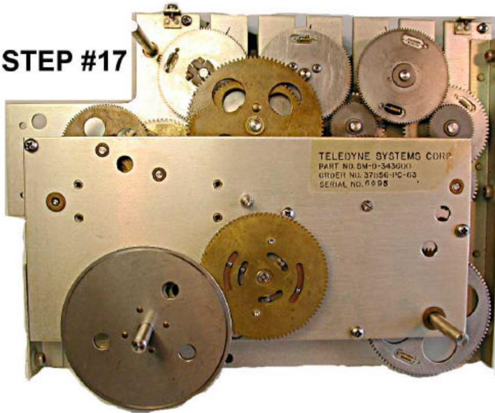
**CLUTCH DISK IS CLAMPED ONTO KHZ SHAFT.**
