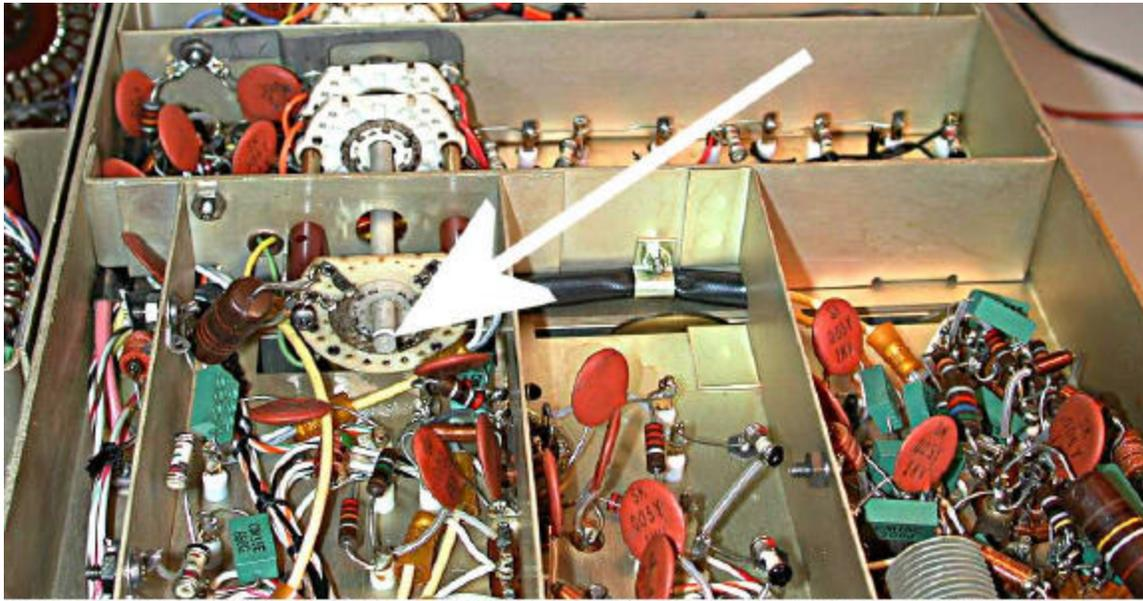
**THIS IS THE WAFER OF THE RF BANDSWITCH THAT WE WILL BE LOOKING AT TO MECHANICALLY ALIGN THIS SWITCH. IT HAS 6 POSITIONS. THE SWITCH CHANGES POSITIONS WHEN THE MHZ DIAL IS CHANGED FROM: 0 TO 1 MHZ, 1 TO 2 MHZ, 3 TO 4 MHZ, 7 TO 8 MHZ AND 15 TO 16 MHZ. NOTE THAT I SAID THAT THESE ARE THE TRANSITIONS AT WHICH THE SWITCH CHANGES. THE 6 SWITCH SETTINGS REPRESENT THE FOLLOWING BANDS: .5 TO 1 MHZ, 1 TO 2 MHZ, 2 TO 4 MHZ, 4 TO 8 MHZ, 8 TO 16 MHZ AND 16 TO 32 MHZ.**
