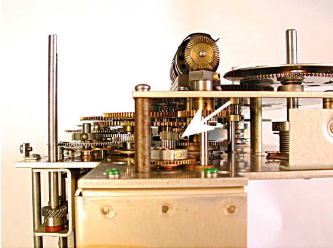
**THIS IS THE CLAMP THAT YOU NEED TO LOOSEN IN ORDER TO ADJUST THE RF BANDSWITCH. THE CLAMP HOLDS THE PINION GEAR AS SHOWN IN ASSEMBLY PICTURE #2. YOU NEED TO HOLD THE LARGE GEAR ATTACHED TO THIS SMALL PINION GEAR AND ONLY TURN THE GENEVA DRIVE TO SET THE RF BANDSWITCH.**
