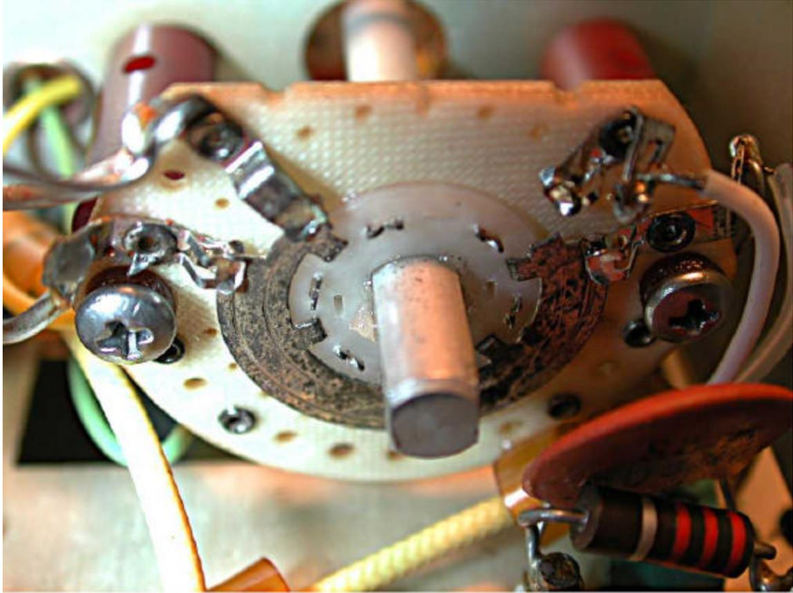
**THIS IS THE POSITION OF THE RF BANDSWITCH REARMOST CONTACTS WHEN THE DIAL IS SET IN THE 07 MHZ POSTION. THE KHZ DIAL HAS NO EFFECT ON THIS SWITCH SETTING.**
