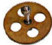
**LUBE SHAFT END AND INSERT WITH SMALL GEAR FACING IN AND MESHING WITH ADJACENT GEAR.**
