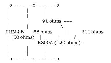
The R390A is seeing 91 ohms in series with approximately 28.45 ohms (the
