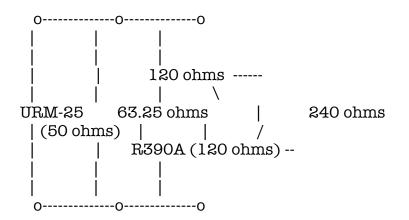
(a 68 Ohm and 910 Ohm in parallel comes close enough to 63.25 Ohms).
