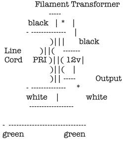
\* Switch the 12 volt leads if output is higher than line!
